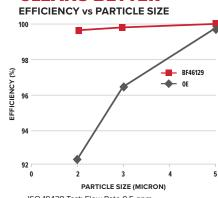
ISO 19438 Test: Flow Rate 0.5 gpm, ISO Medium Test Dust, 104°F, Termination at 6 psid
