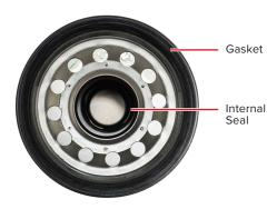
**Note:** A thin layer of clean motor oil must be applied to the gasket and internal seal before installing the filter. Applying oil to the internal seal will allow the internal seal to slide onto the post on the filter mounting base.
