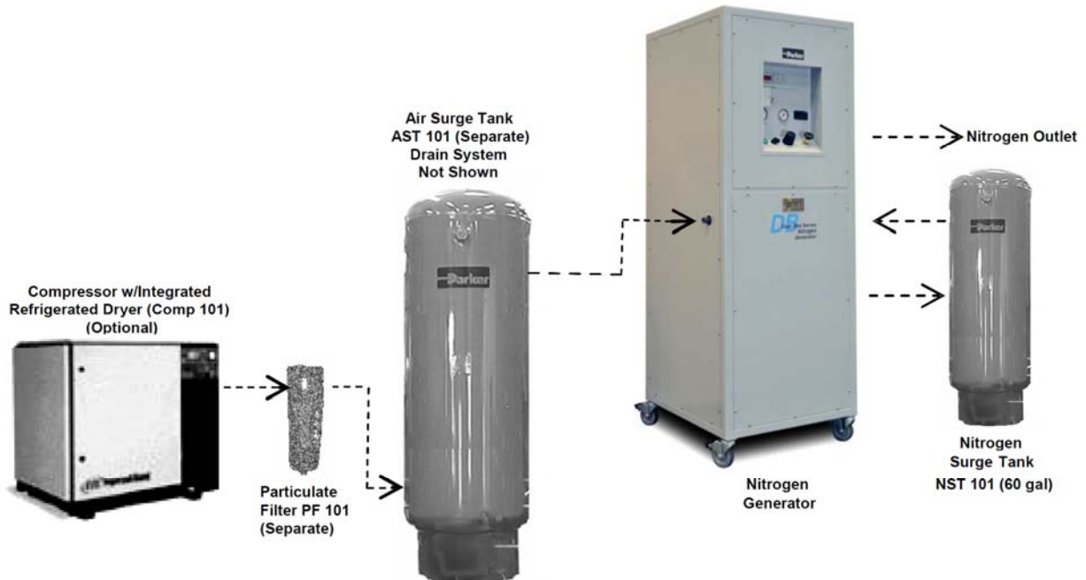
Figure 1: Typical Setup of the Parker Dual Bed Nitrogen Generator
