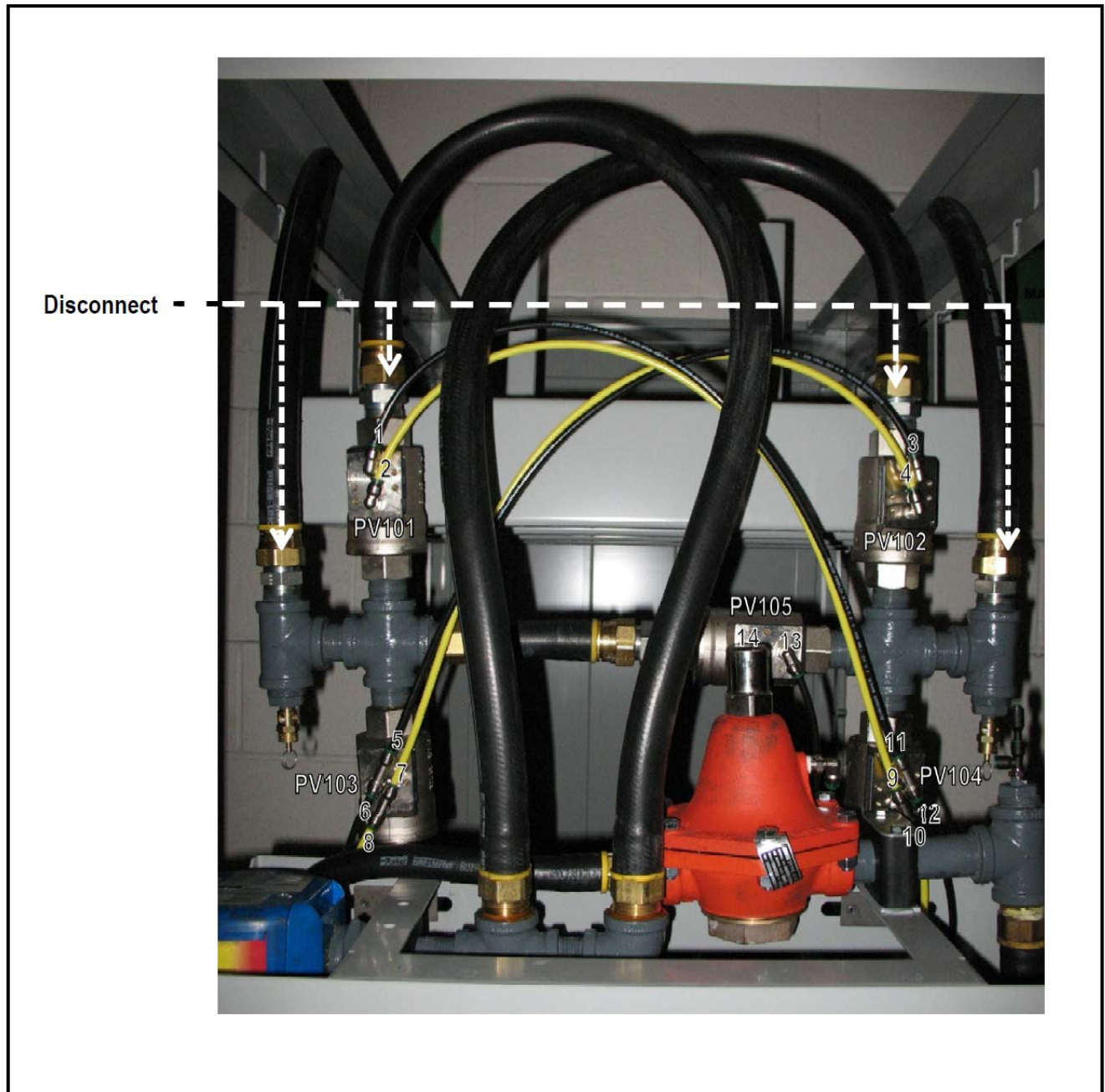
Figure 12: AGS500/600 Top Manifold - Label All Tubing Connections
