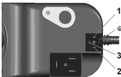
Type C plug: potential-free contact
