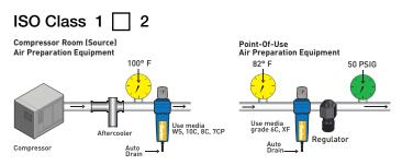
Any compressor with aftercooler and 2-stage coalescing. Air intended for use with lubricated control valves, cylinders, parts blow-down, etc.
