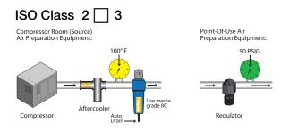
Any compressor with aftercooler. Air intended for use with lubricated air tools, air motors, cylinders, shot blasting, non-frictional valves.
