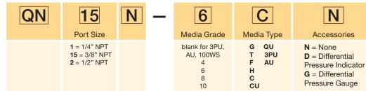
For Example: QN15N-10QUN for complete assembly, including element. QN15NN X 1 for an empty housing. Mounting bracket: P/N BK-M Note: Although the element size is not included in the part number construction for this filter, the size, 10-025, is needed to order replacement elements. For Example, 6C10-025 X 8.
