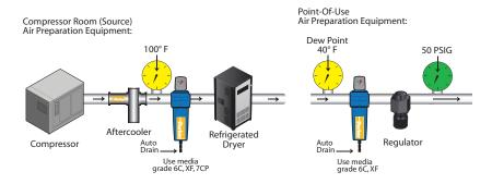
Any compressor with after-cooler, 2-stage coalescing and refrigerated dryer. Air intended for use with air gauging, air conveyors, spraypainting, food processing, instrumentation, blow molding, cosmetics, film processing, bottling, pharmaceuticals, dairy, breweries, medical, robotics and close tolerance valves.
