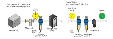
Any compressor with after-cooler, 2-stage coalescing, refrigerated dryer and carbon absorber. Air intended for use as industrial breathing air and decompression chambers. CAUTION: Always use high temperature synthetic lubricants and monitor (alarm for carbon monoxide concentrations). This system will not eliminate toxic gases!
