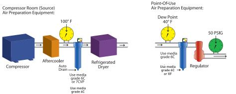
Any compressor with after-cooler, 2-stage or 7CVP, XF refrigerated dryer. Air intended for use with air gauging, air conveyors, spraypainting, food processing, instrumentation, blow molding, cosmetics, film processing, bottling, pharmaceuticals, dairy, breweries, medical, robotics and close tolerance valves.
