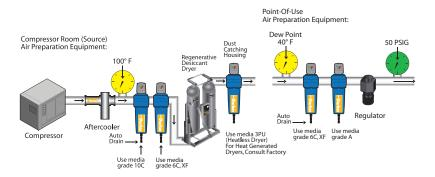
Any compressor with after-cooler, two-stage and double coalescing regenerative-type desiccant dryer and a carbon adsorber. Air intended for use in applications involving rapid expansion of compressed air, critical instrumentation, high purity gases, automotive paint systems, etc. CAUTION: This air is too dry for respiratory use.
