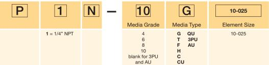
For Example: P1N-4QU10-025 for complete assembly, including element. P1N X 1 for an empty housing. **Mounting Bracket**: MB-2
