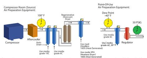
Any compressor with after-cooler, two-stage and double cruise media and a regenerative-type desiccant dryer. Air intended for use in applications involving rapid expansion of compressed air, critical instruing grade 6C, XF high purity gases, computer chip drying, etc.
