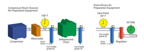
Any compressor with after-cooler, 2-stage coalescing and deliquescent dryer. Air intended for use with general pneumatic systems, body shop spray painting and components sensitive to high moisture content.
