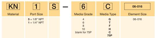
For Example: KN1S-6C06-016 for complete assembly, including element. KN1S X 1 for an empty housing. **Mounting Bracket**: MBS-2
