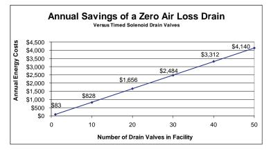
The annual cost of compressed air was calculated using data from the U.S. Department of Energy and several compressed air consultants. The average annual energy cost to maintain a compressed air system is \$0.23 per 1000 ft<sup>3</sup>. If a timed solenoid drain valve opens 3-4 times per hour, the cost of the wasted air will be \$80 per valve, per year.
