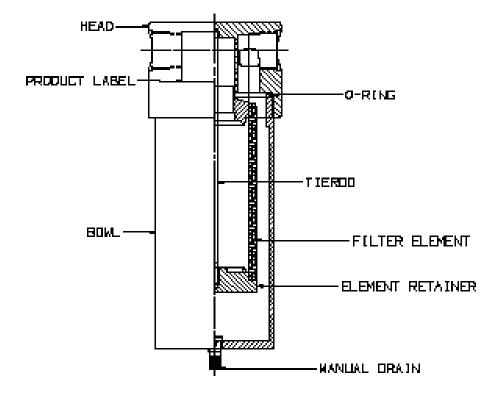
Figure 2 - Drain Details
