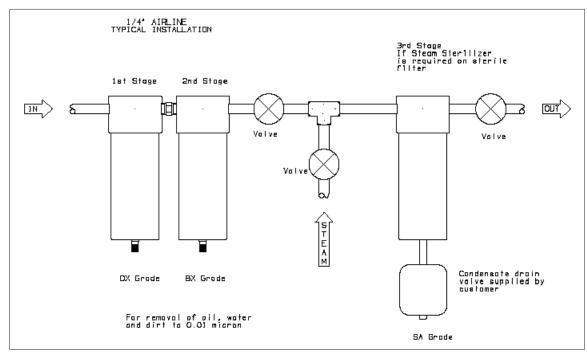
Figure 4 - Schematic Installation
