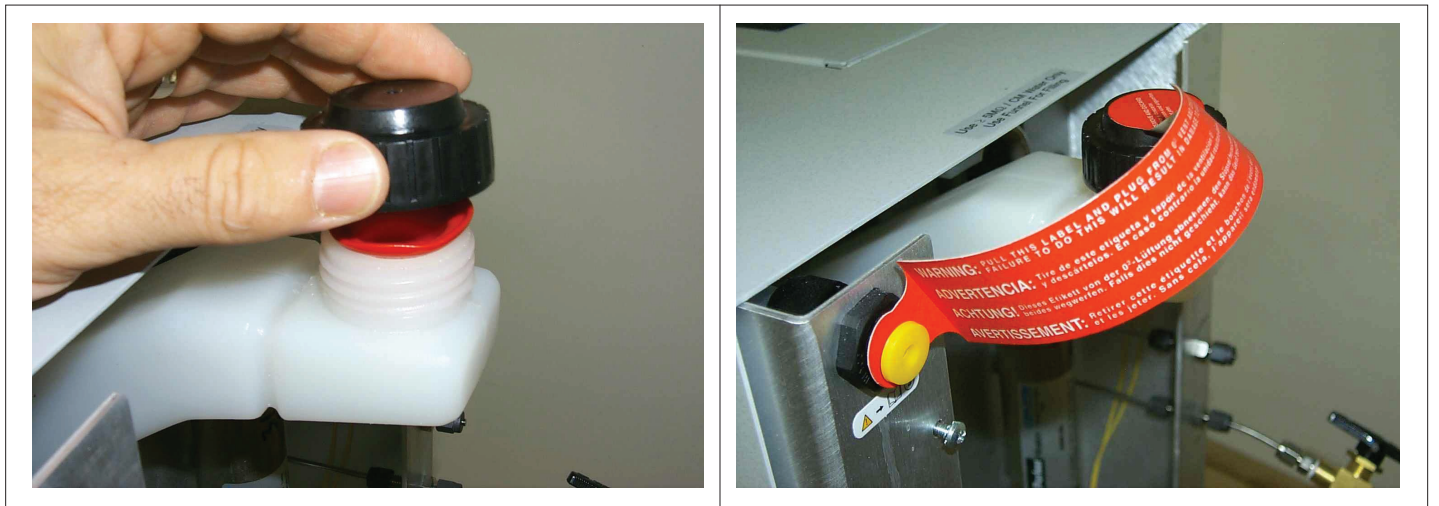
C. Install yellow plug in vent tube and stick label over cap vent as shown
